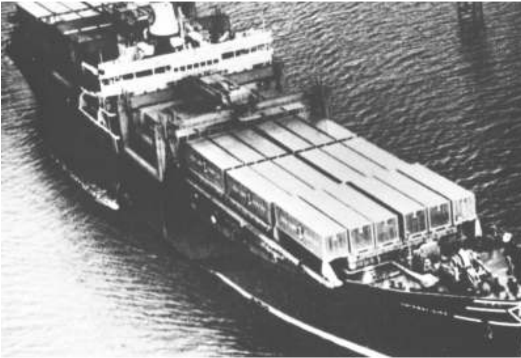
The Gateway City, modified into the first cellular container ship in 1957. Shipboard gantry cranes have been installed to handle the containers ship to shore
