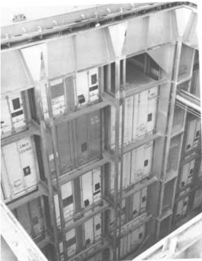
CML's cell guides of their container ships in the early 60's
