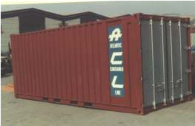
The first “rust brown” MAFI Steel Container with the “flat panel” for a company’s logo and container marking
