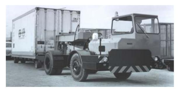
A platform with detachable goose neck and a tractor with the goose neck hitched to an elevating fifth wheel. This concept was first documented on 22 February 1966 and became a patent for MAFI in June 1969 with Ulrich Cramer as inventor.
